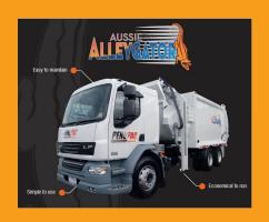
Designed for alleyways and tight area collections and with the lifting capacity of 280kg, the Pendpac Aussie Alleygator is an innovation in solid waste collection technologies. It's developers Neville Farrugia and Michael Thobe from Twin City Truck Centre in Albury Woodonga made contact with ICN early on to discuss establishing local supply chains and import replacement opportunities.
