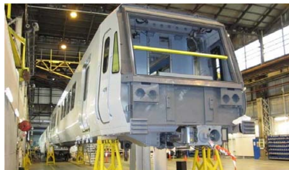
X'Trapolis train on the assembly line
